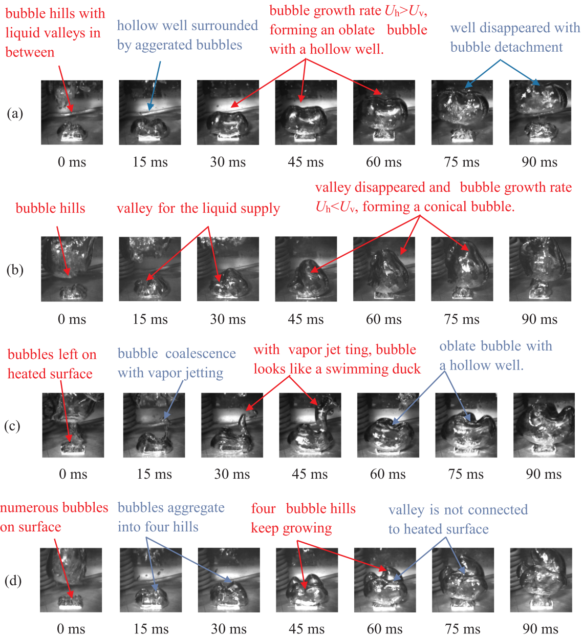
Fig. 11. Bubble dynamics corresponding to the cases of the maximum heat transfer coefficient for different surfaces. (a) BS, q = 980.4 \text{ kW/m}^2 ; (b) TS1, q = 1617.8 \text{ kW/m}^2 ; (c) TS2, q = 1549.8 \text{ kW/m}^2 ; (d) TS3, q = 1295.1 \text{ kW/m}^2 .
