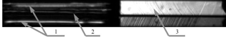
Figure 3. Air–water calibration result in a single microchannel. 1: Liquid film in the corner; 2: gas core (air); 3: liquid plug.
