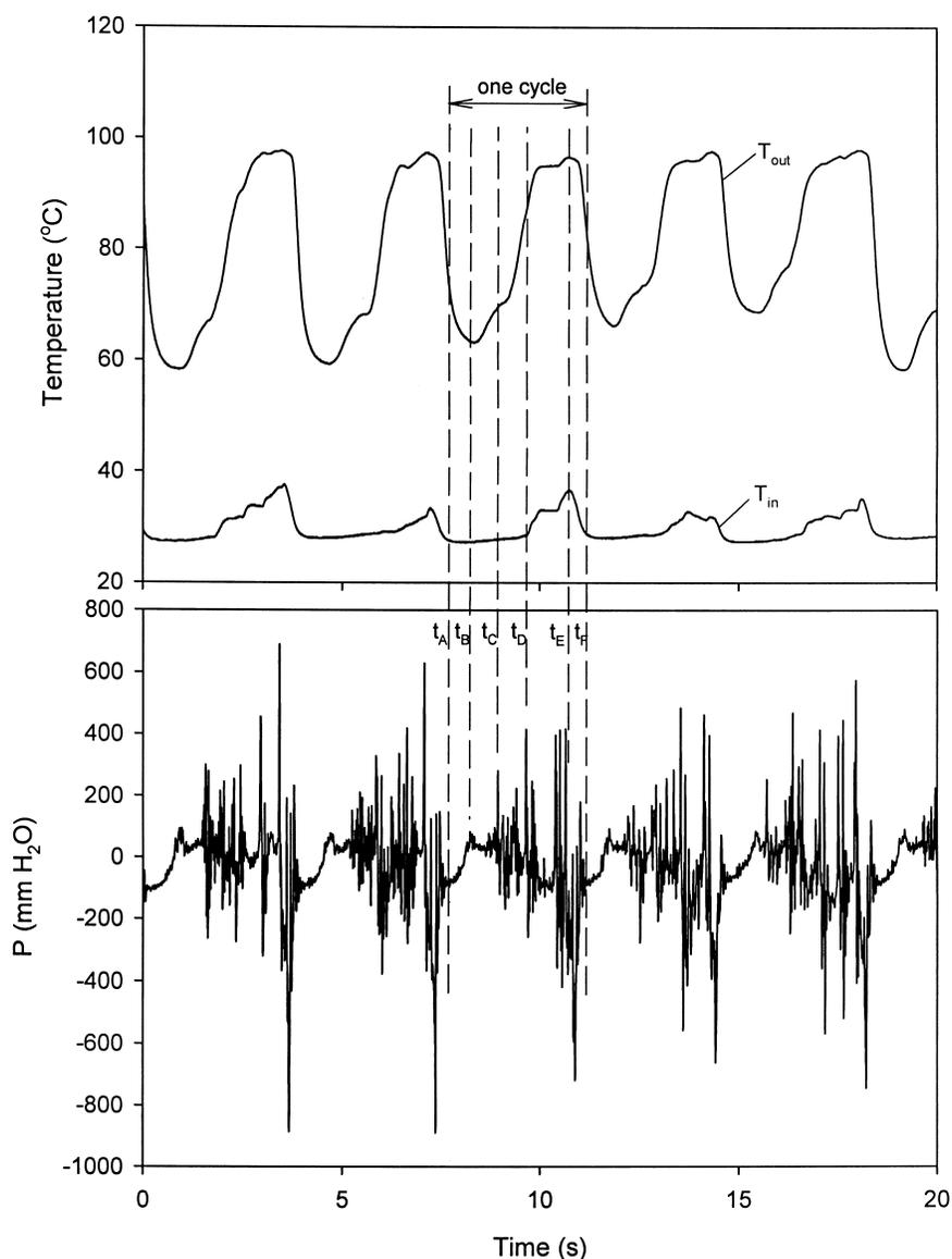
Figure 5. Dynamic measurements of the heat driven pump at the heating power of 20 W.
