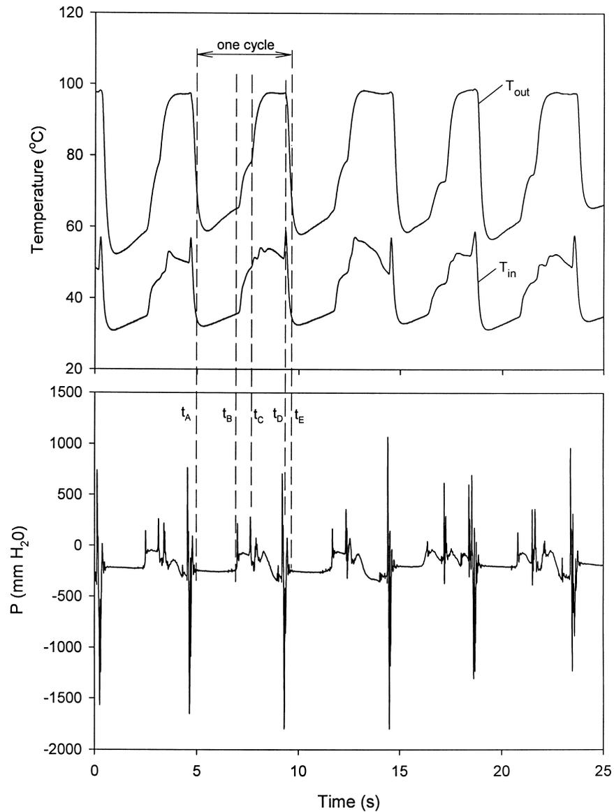
**Figure 8.** Dynamic measurements of the inverted U-shaped heat driven pump at the heating power of 20 W.
