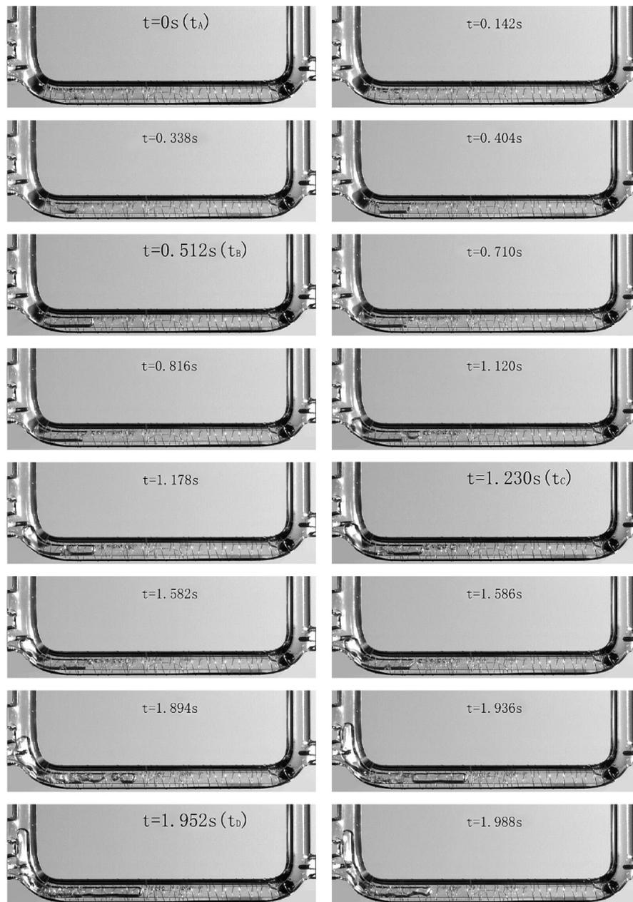
**Figure 6.** High-speed flow visualization of the U-shaped heat driven pump at the heating power of 20 W (*continues*).
