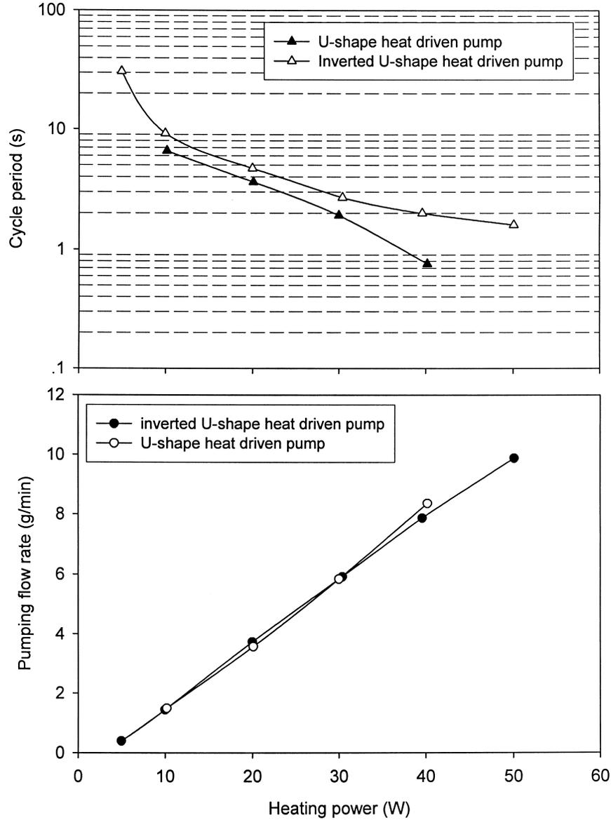
Figure 10. Cycle periods and pumping flow rates for both heat driven pumps.
