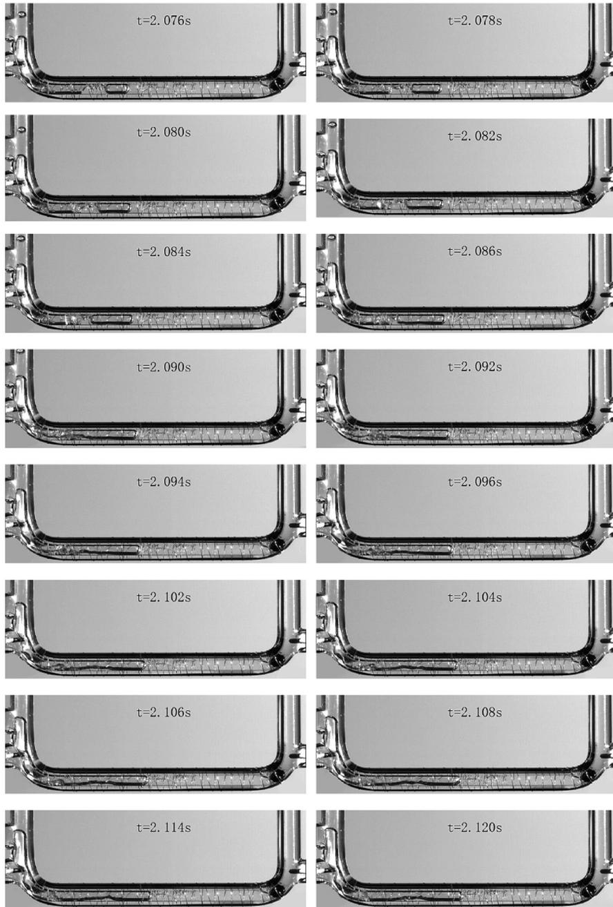
**Figure 7.** The successive images illustrating the formation of the wave vapor/liquid interface on the bottom of the capillary tube.
