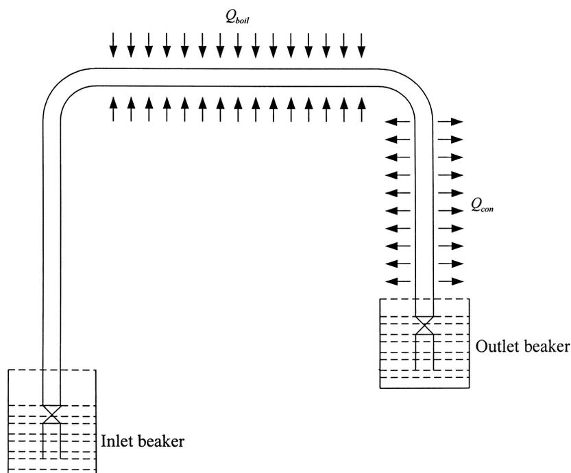
Figure 11. Ideal heat driven pumps demonstrating the working principles.
