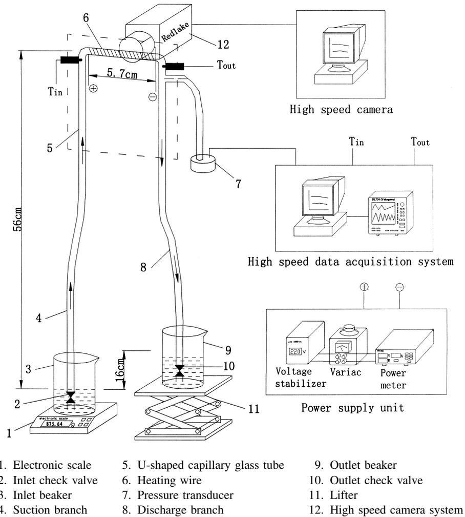
Figure 2. Experimental setup of the inverted U-shaped heat driven pump.
