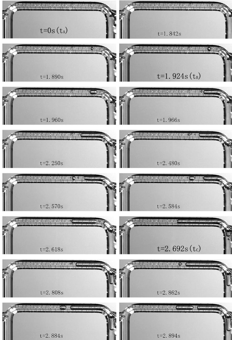
**Figure 9.** High-speed flow visualization of the inverted U-shaped heat driven pump at the heating power of 20 W (*continues*).
