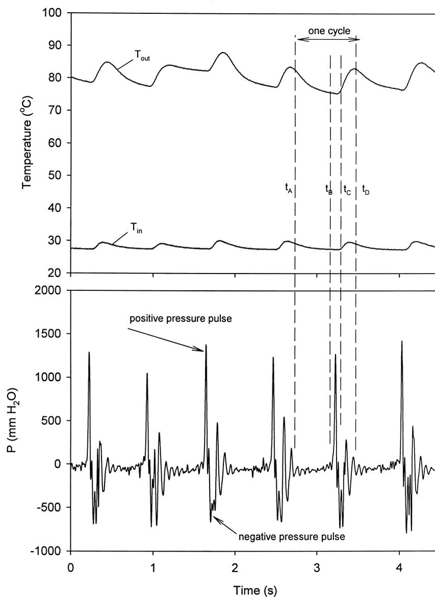
**Figure 3.** Dynamic recordings of pressures and fluid temperatures versus time for the U-shaped heat driven pump at the heating power of 40.0 W.
