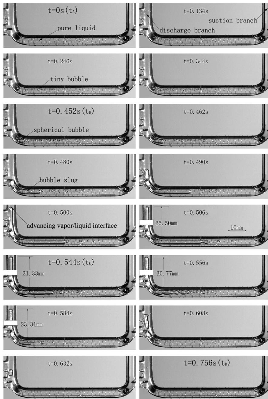
Figure 4. High-speed flow visualization of the U-shaped heat driven pump at the heating power of 40 W.
