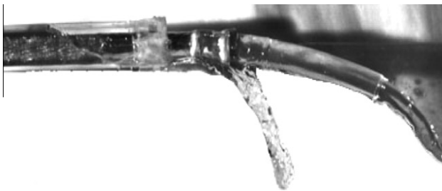
Fig. 13. Image at the mesh cylinder outlet and annular region for intermittent flow pattern.
