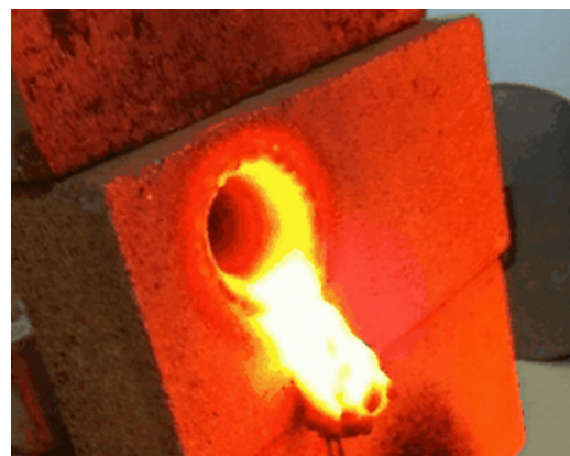
Fig. 3 A refractory brick is being melt by the solar simulator, the melting temperature of the brick is about 2300 K
